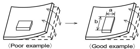
(2) Components location on PCB separation
