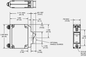
Note: Tolerance ± .015 [.38] unless noted. Dimensions in brackets [] are millimeters.
