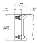
NOTE: THIS BARRIER CAN BE FLIPPED TO COVER EITHER POLE. PLEASE CONTACT FACTORY FOR SPECIFIC PART NUMBER
