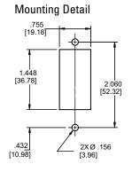
Panel Mounting Detail Tolerance ±.005 [.13] unless noted.
