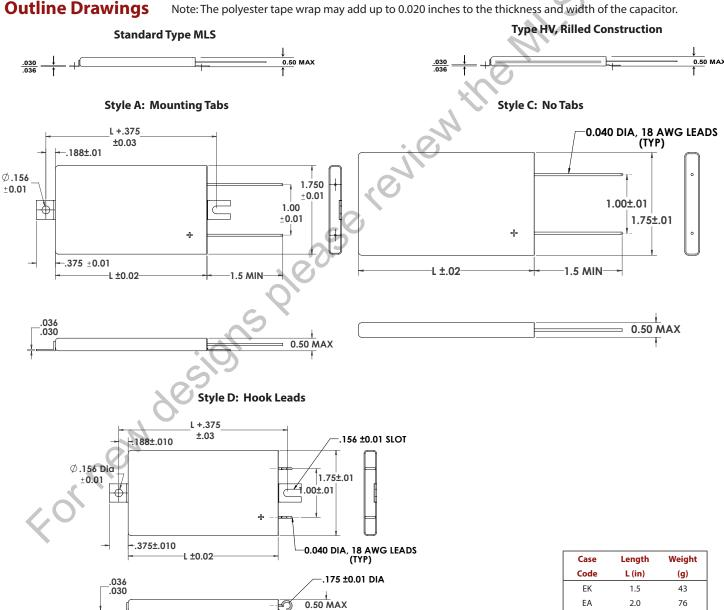
Mounting tabs are welded to the case.
