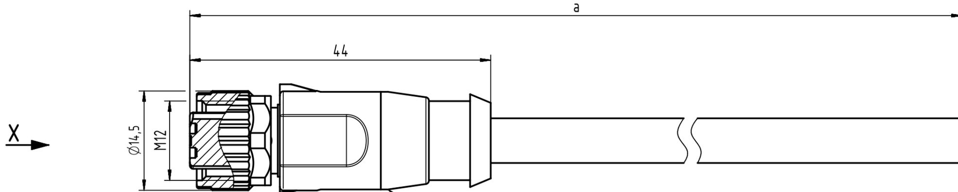
M12 D-coded 4 poles, straight overmolded female connector
