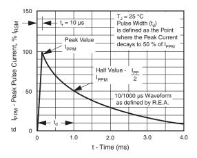
Fig. 3 - Pulse Waveform
