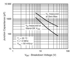
Fig. 4 - Typical Junction Capacitance
