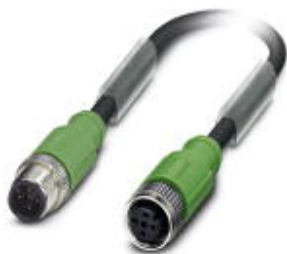
Sensor/actuator cable, 4-position, PUR halogen-free, black-gray RAL 7021, shielded, Plug straight M12, A-coded, on Socket straight M12, A-coded, cable length: 10 m
