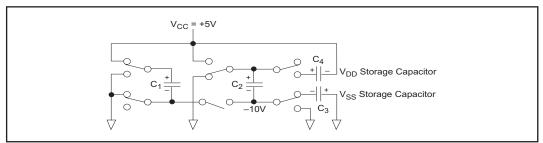
Figure 3, Charge pump - Phase 2
