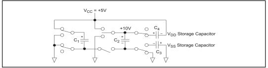
Figure 5, Charge pump - Phase 4
