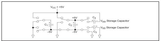
Figure 4, Charge pump - Phase 3
