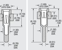
Contact Length = (2.11 mm) .083" Lead DIA Accepted = (0.38 mm) .015" to (0.51 mm) .020" Insertion Denth = (2.67 mm) .105" to (4.32 mm) .170" Style 10 Component Part No. = SC-3P1
