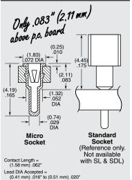
Insertion Depth = (1.65 mm) .065" to (3.56 mm) .140"
