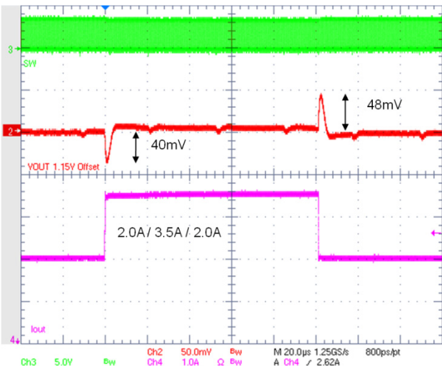
Figure 32. Transient Load 2.0 – 3.5 A Auto Mode
