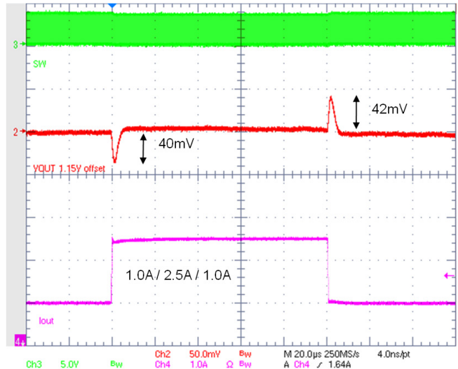
Figure 31. Transient Load 1.0 – 2.5 A Forced PWM Mode
