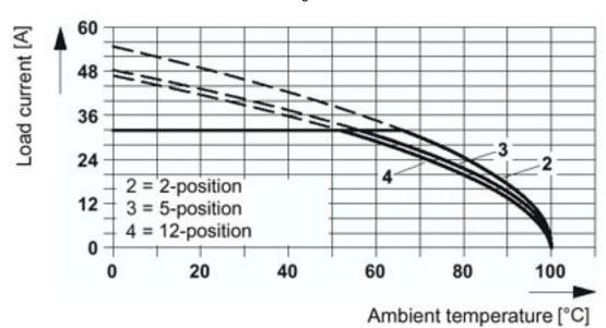
The illustration shows the derating curve for plugs PC 5/...-ST-7,62 in combination with header PC 4/...-G-7,62.
