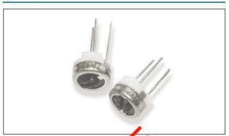
For applications that demand a durable, miniature tria ming potentiometer, this military style offers quality at the right price. Cermes element technology ensures stability and performance in these 6mm diameter components. All buts are fully sealed to withstand immersion in normal board washing solvents.
