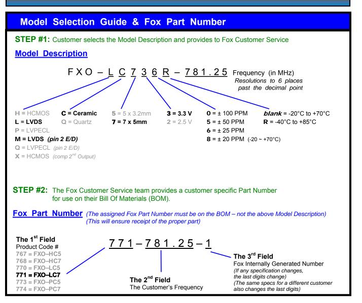
This example, FXO-LC736R-781.25 = LVDS Output, Ceramic, 7 x 5mm Package, 3.3V, ±25 PPM Stability, -40 to +85°C Temperature Range, at 781.25 MHz
