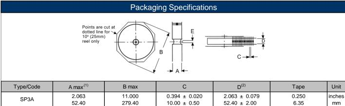
Dimension "E": This is a non-critical dimension that does not have a tolerance in the standard. Range of diameters is from 0.547 inches (13.90 mm) to 1.500 inches (38.10 mm).
