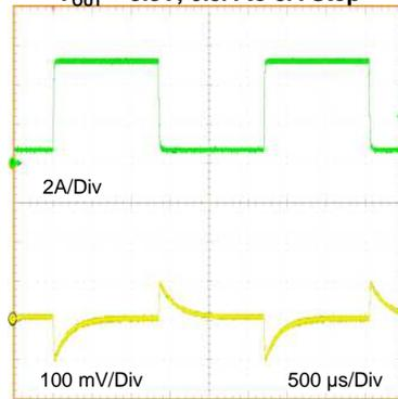
**LMZ23603 Load Step Response  $V_{IN} = 12V$
