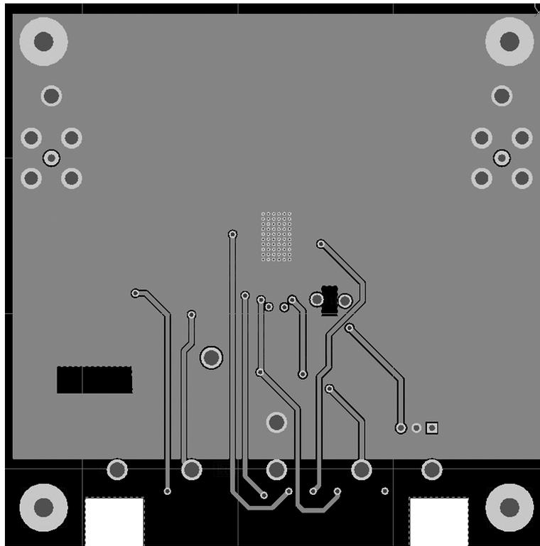
**Figure 5. Internal Layer II (Ground and Routing)
