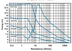
These graphs are irregular owing to the necessity to adapt the commercial dimension of wire to the resistance range, however they are enough to show the trend of this characteristic.
