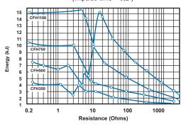
Absorbed energy for wire temperature of 800°C (Impulse time ≤ 0.2")
