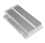
The CFH is a high quality range of aluminium housed power resistors offering environmental protection to IP55, 6kV dielectric strength, 1.8kW power dissipation, and the ability to absorb electrical pulses of up to 24kJ.
