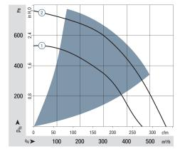
Air performance measured according to: ISO 5801. Installation category A, with ebm-papst inlet ring without contact protection.
