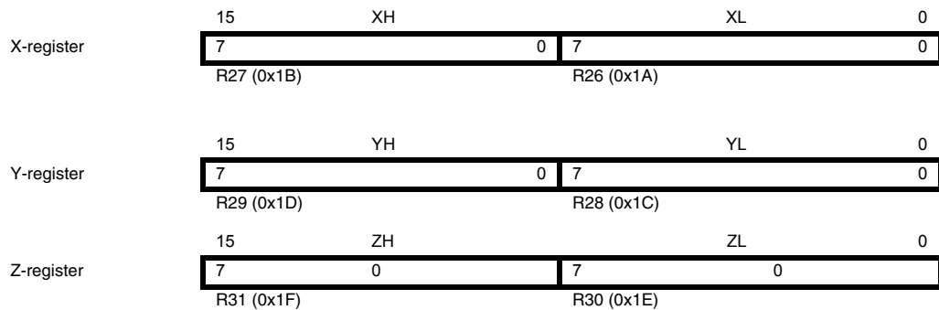
Figure 7-3. The X-, Y-, and Z-registers
