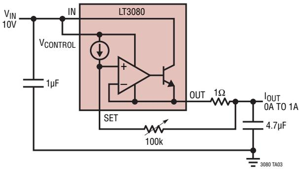
Low Dropout Voltage LED Driver
