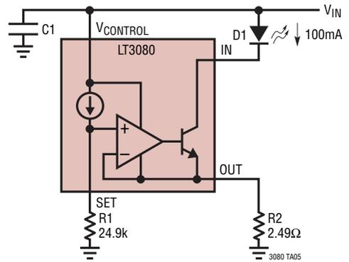
Using a Lower Value SET Resistor
