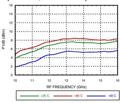
Output P1dB, USB vs. Temperature
