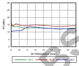
Output IP3, USB vs. Temperature
