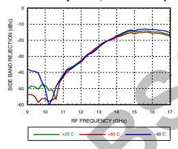
Input P1dB, USB vs. Temperature
