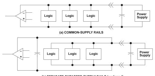
(b) SEPARATE-BYPASSED SUPPLY RAILS (preferred)
