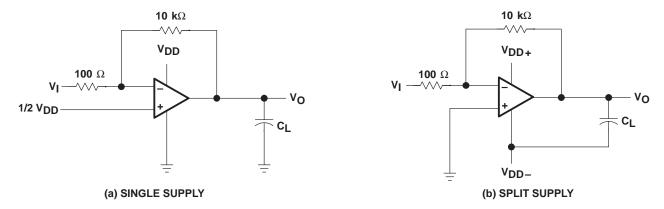
Figure 36. Gain-of-100 Inverting Amplifier
