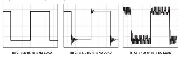
Figure 45. Effect of Capacitive Loads
