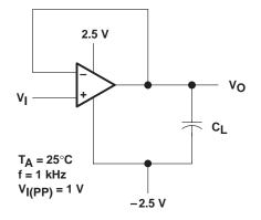
Figure 44. Test Circuit for Output Characteristics
