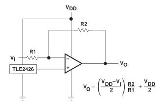
Figure 39. Inverting Amplifier With Voltage Reference
