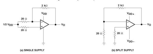
Figure 35. Noise-Test Circuit
