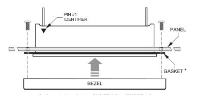
\*Sealing gasket is optional on DMS-BZL2-C and DMS-BZL4-C  $\,$
