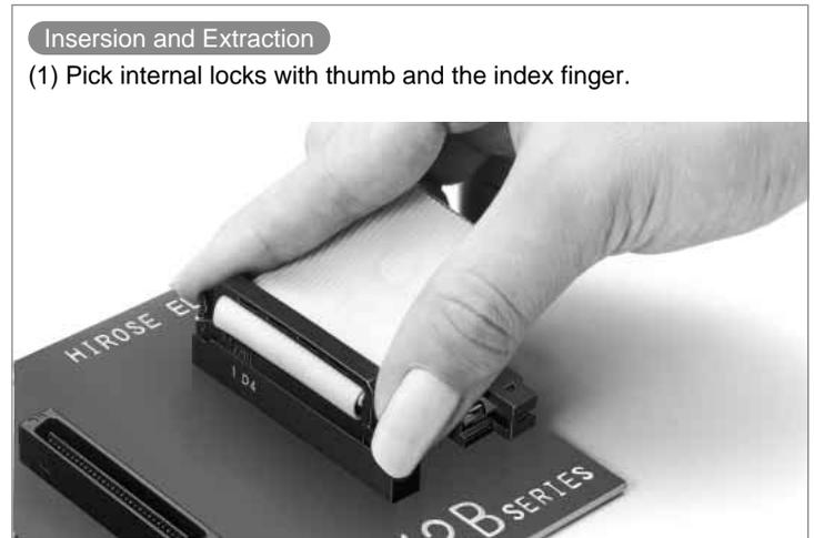
(2) With unique and preferable click feeling, the cable and connector can be inserted or withdrawn.
