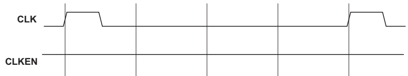
Figure 5-2 Stopping CLK for power saving
