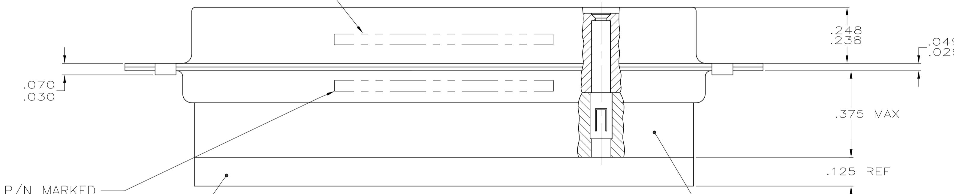
6 FOR (-1 & -11) CUSTOMER P/N MARKED ON FAR SIDE. MANUFACTURER'S NAME, BRAND OR LOGO AND MANUFACTURER'S PART NO AND DATE CODE MARKED ON NEAR SIDE. FOR(-2, -4 & -7) MARK MFG'S P/N FAR SIDE.
