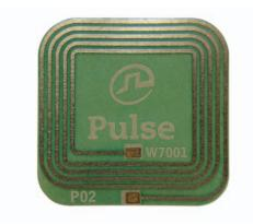
The W7001 is a small flexible Near Field Communication (NFC) antenna ideal for embedded products such as tablets, laptops, and payment terminal devices. It is intended for both secure payment or security access applications.
