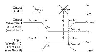
Voltage Waveform Enable and Disable Times
