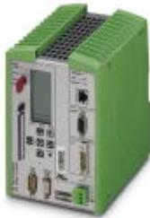
Remote Field Controller with 1x10/100 Ethernet, INTERBUS-Master, IP20 degree of protection, pluggable parameterization memory (MC FLASH)
