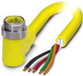
Sensor/actuator cable, 5-position, PVC, yellow, Plug angled 7/8"-16UNF, A-coded, on free cable end, cable length: 6 m
