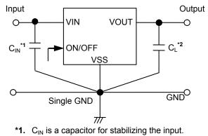
\*2. A ceramic capacitor of 0.1  $\mu$ F or more can be used as C<sub>L</sub>.
