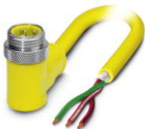
Sensor/actuator cable, 3-position, PVC, yellow, Plug angled 7/8"-16UNF, A-coded, on free cable end, cable length: 2 m
