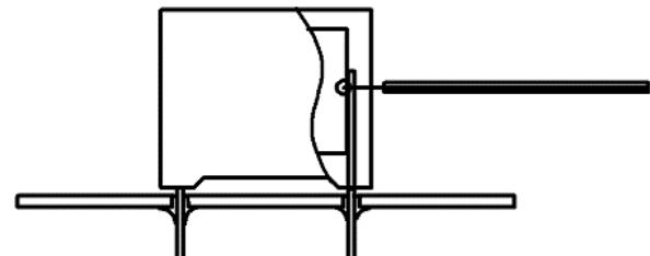
The temperature is monitored inside the capacitor.
