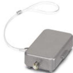
HEAVYCON protective cover, type B10, for supporting base element with single locking latch, with retaining cord, IP65, ALU
