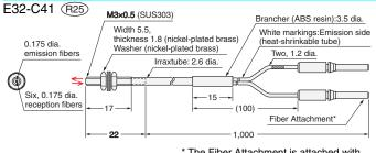
\* The Fiber Attachment is attached with adhesive and cannot be removed.
