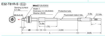
Note: The maximum allowable temperatures for sections A and B are 200°C and 110°C, respectively. The section inserted into the Amplifier Unit (indicated by \*), however, must stay within the Amplifier Unit's operating temperature range.
