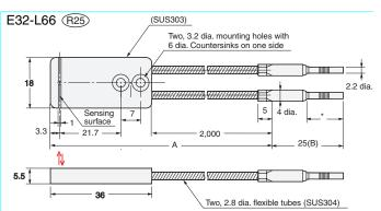
Note: The maximum allowable temperatures for sections A and B are 300°C and 110°C, respectively. The section inserted into the Amplifier Unit (indicated by \*), however, must stay within the Amplifier Unit's operating temperature range.
