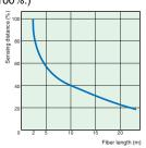
Fiber Units with Reflective Sensors (Fiber length of 2 m corresponds to 100%.)
