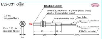
Note: There is a white line on the cable fiber that is inserted in the emitter-side port.
