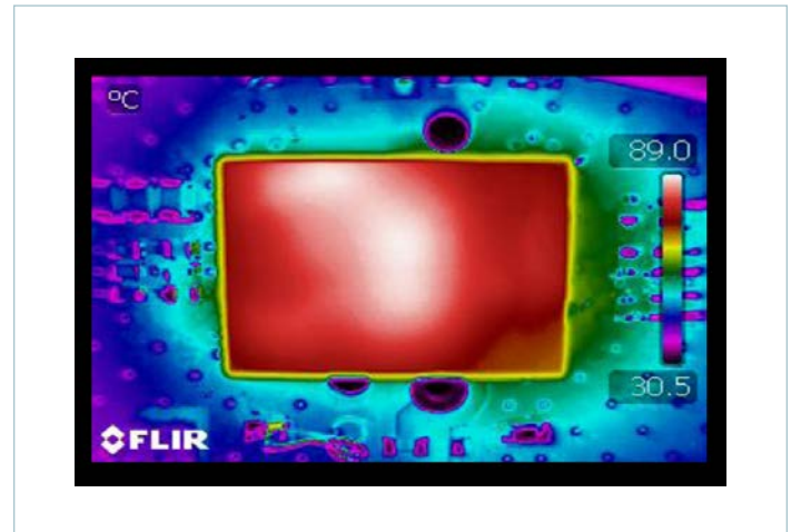
Figure 20 — Thermal image ( V_{IN} = 48V , I_{OUT} = 5A , CR, OLFM evaluation PCB)
