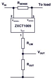
ZXCT1009 with additional current limiting Resistor R<sub>LIM</sub>.
