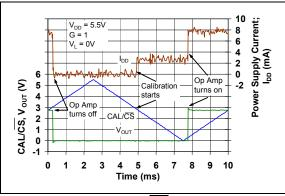
**FIGURE 2-46:** CAL $\overline{/CS}$  Voltage, Output Voltage and Supply Current (for Side A) vs. Time with  $V_{DD} = 5.5V$ .
