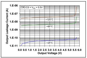
**FIGURE 2-51:** Output Leakage Current vs. Output Voltage.
