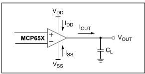
**FIGURE 4-8:** Diagram for Capacitive Load Power Calculations.
