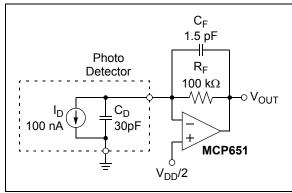
**FIGURE 4-14:** Transimpedance Amplifier for an Optical Detector.
