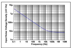
FIGURE 2-32: Input Noise Voltage Density vs. Frequency.
