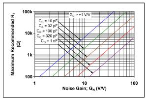
**FIGURE 4-12:** Maximum Recommended  $R_F$  vs. Gain.
