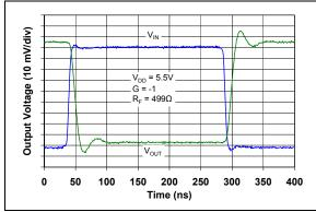
**FIGURE 2-39:** Inverting Small Signal Step Response.
