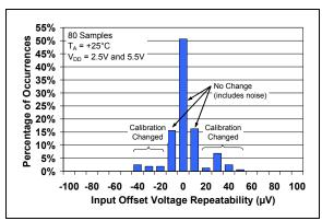
**FIGURE 2-3:** Input Offset Voltage Repeatability (repeated calibration).
