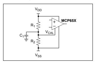
**FIGURE 4-2:** Setting V<sub>CM</sub> with External Resistors.
