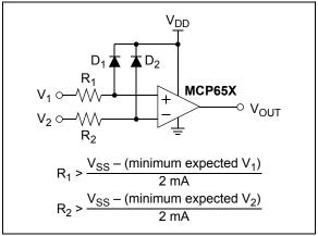
FIGURE 4-4: Protecting the Analog Inputs.
