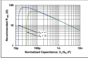
**FIGURE 4-10:** Recommended R<sub>ISO</sub> Values for Capacitive Loads.
