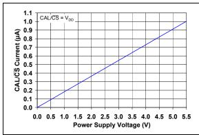
FIGURE 2-44: CAL/CS Current vs. Power Supply Voltage.
