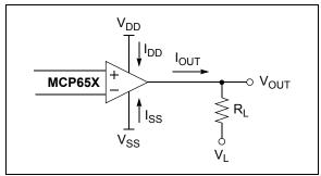
**FIGURE 4-7:** Diagram for Resistive Load Power Calculations.
