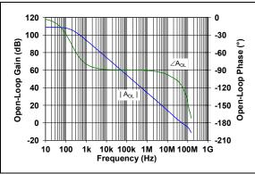
FIGURE 2-25: Open-Loop Gain vs. Frequency.
