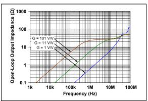
FIGURE 2-29: Closed-Loop Output Impedance vs. Frequency.
