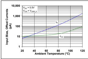
**FIGURE 2-12:** Input Bias and Offset Currents vs. Ambient Temperature with  $V_{DD} = +5.5V$ .
