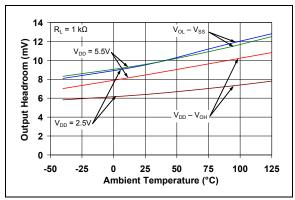
**FIGURE 2-17:** Output Voltage Headroom vs. Ambient Temperature.
