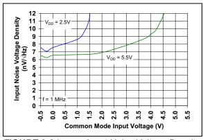
**FIGURE 2-34:** Input Noise Voltage Density vs. Input Common Mode Voltage with f = 1 MHz.
