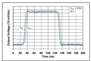
FIGURE 2-37: Non-inverting Small Signal Step Response.
