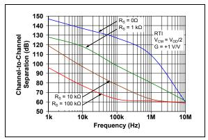
FIGURE 2-31: Channel-to-Channel Separation vs. Frequency.
