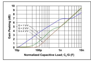
**FIGURE 2-30:** Gain Peaking vs. Normalized Capacitive Load.
