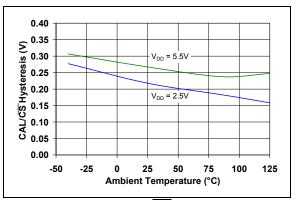
**FIGURE 2-47:** CAL/CS Hysteresis vs. Ambient Temperature.
