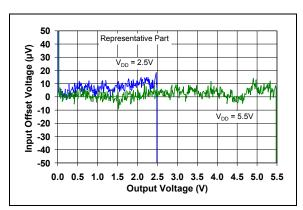
**FIGURE 2-5:** Input Offset Voltage vs. Output Voltage.
