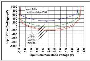
**FIGURE 2-9:** Input Offset Voltage vs. Common Mode Voltage with  $V_{DD} = 5.5V$ .
