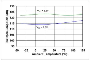
**FIGURE 2-11:** DC Open-Loop Gain vs. Ambient Temperature.
