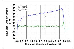
**FIGURE 2-13:** Input Bias and Offset Currents vs. Common Mode Input Voltage with  $T_A = +85$ °C.
