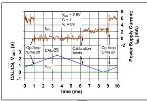
**FIGURE 2-45:** CAL/ $\overline{CS}$  Voltage, Output Voltage and Supply Current (for Side A) vs. Time with  $V_{DD}$  = 2.5V.
