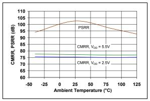
**FIGURE 2-10:** CMRR and PSRR vs. Ambient Temperature.
