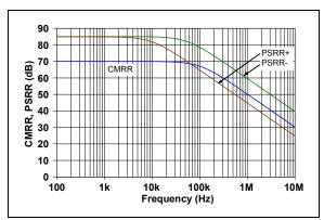
**FIGURE 2-24:** CMRR and PSRR vs. Frequency.
