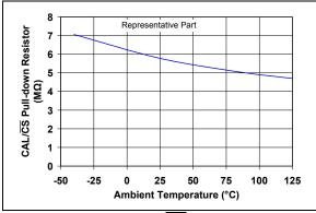
**FIGURE 2-49:**  $CAL/\overline{CS}$ 's Pull-down Resistor ( $R_{PD}$ ) vs. Ambient Temperature.
