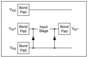
FIGURE 4-3: Simplified Analog Input ESD Structures.
