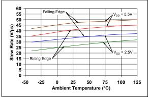
**FIGURE 2-42:** Slew Rate vs. Ambient Temperature.
