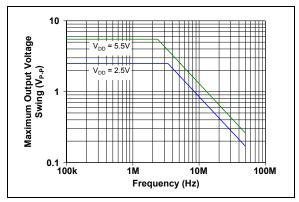
FIGURE 2-43: Maximum Output Voltage Swing vs. Frequency.
