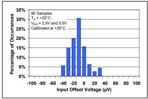
FIGURE 2-1: Input Offset Voltage.
