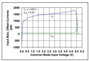
**FIGURE 2-14:** Input Bias and Offset Currents vs. Common Mode Input Voltage with  $T_A = +125$ °C.
