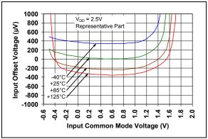
**FIGURE 2-8:** Input Offset Voltage vs. Common Mode Voltage with  $V_{DD} = 2.5V$ .
