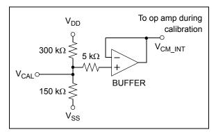
FIGURE 4-1: Common-Mode Reference's Input Circuitry.
