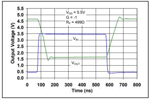
**FIGURE 2-40:** Inverting Large Signal Step Response.
