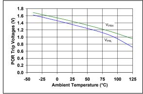
**FIGURE 2-21:** Power On Reset Voltages vs. Ambient Temperature.
