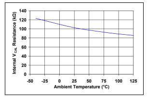
**FIGURE 2-23:** V<sub>CAL</sub> Input Resistance vs. Temperature.
