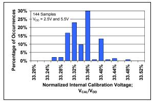
FIGURE 2-22: Normalized Internal Calibration Voltage.
