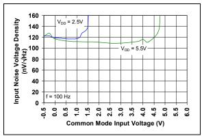
**FIGURE 2-33:** Input Noise Voltage Density vs. Input Common Mode Voltage with f = 100 Hz.
