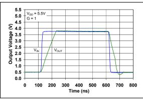
FIGURE 2-38: Non-inverting Large Signal Step Response.
