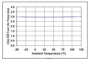
**FIGURE 2-48:** CAL/CS Turn On Time vs. Ambient Temperature.
