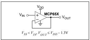
FIGURE 4-5: Unity Gain Voltage Limitations for Linear Operation.
