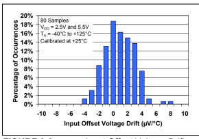
FIGURE 2-2: Input Offset Voltage Drift.
