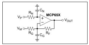
**FIGURE 4-11:** Amplifier with Parasitic Capacitance.
