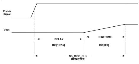
Fig. 20: Channel Power Up Sequence
