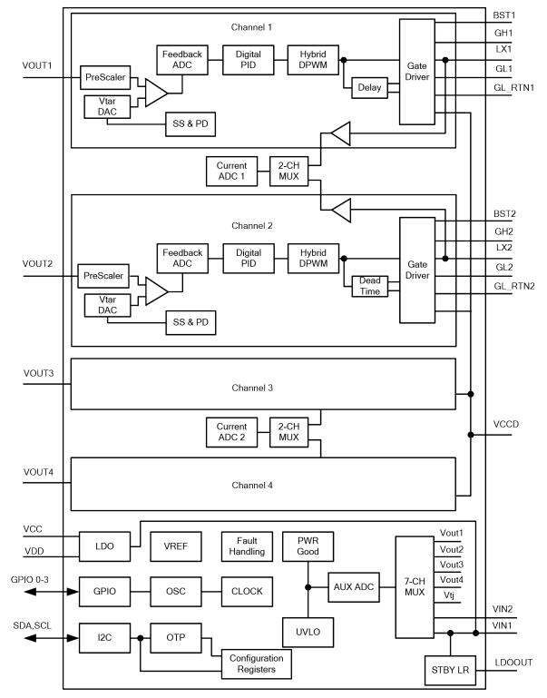
Fig. 2: XRP7740 Block Diagram
