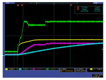
Fig. 18: VCCA (green) Startup Waveform
