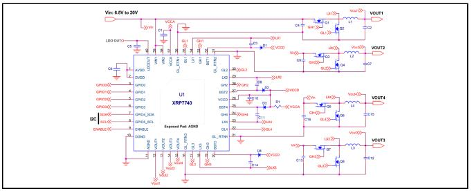
Fig. 1: XRP7740 Application Diagram
