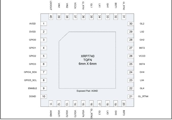
Fig. 3: XRP7740 Pin Assignment
