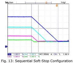
Vout Shutdown = 0.8V, No Load CH1:3.3V CH2:5V CH3:1V CH4:1.8V
