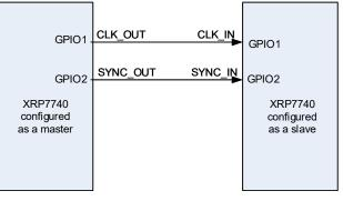
Fig. 24: Master/Slave Configuration of the XRP7740
