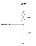
Fig. 17: RC Delay for Enable taken from VCCA
