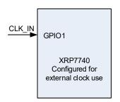
Fig. 23: XRP7740 Configured For External Clock Use
