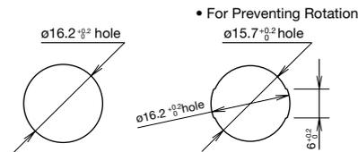
\* Chamfering on the front edge of the mounting hole is recommended for easy insertion.
