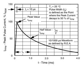
Fig. 3 - Pulse Waveform
