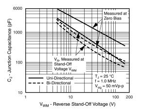
Fig. 4 - Typical Junction Capacitance
