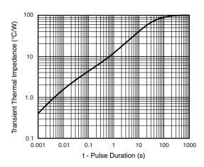
Fig. 5 - Typical Transient Thermal Impedance
