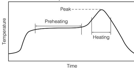
For soldering (Example : Sn/Pb)
