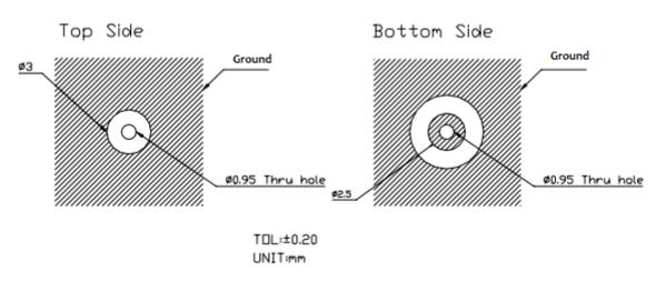
\*Note Layout Dimensions may be affected by the thickness of the PCB
