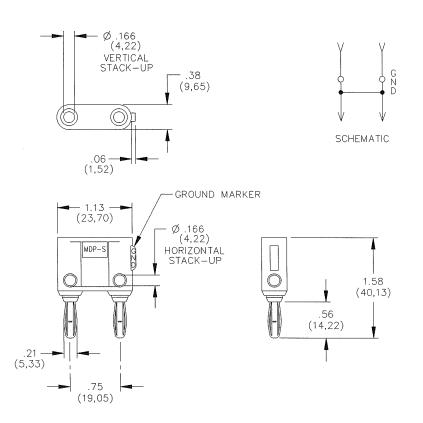
MATERIALS: Body – Nickel Plated Brass Contacts – Nickel Plated Beryllium Copper Insulator – Nylon
