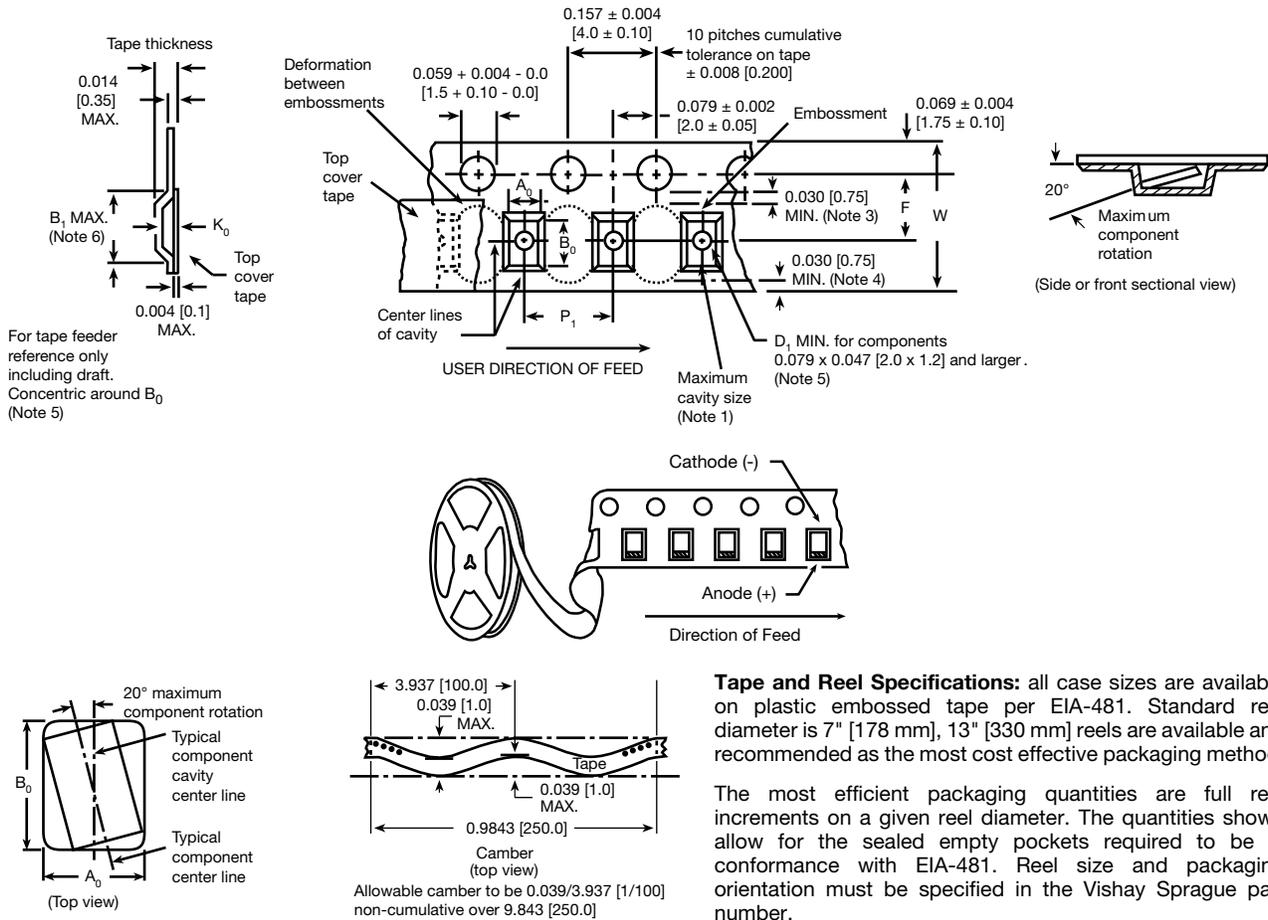
**Tape and Reel Specifications:** all case sizes are available on plastic embossed tape per EIA-481. Standard reel diameter is 7" [178 mm], 13" [330 mm] reels are available and recommended as the most cost effective packaging method.
