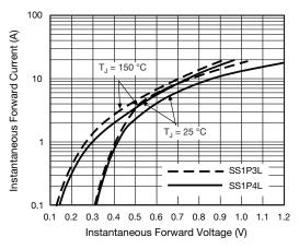
Fig. 3 - Typical Instantaneous Forward Characteristics
