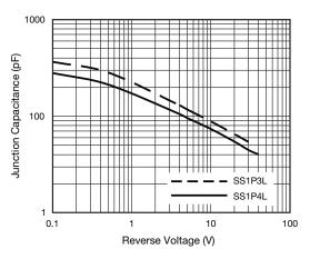
Fig. 5 - Typical Junction Capacitance
