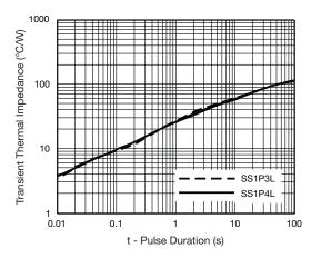
Fig. 6 - Typical Transient Thermal Impedance
