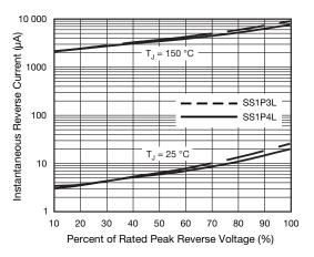
Fig. 4 - Typical Reverse Leakage Characteristics
