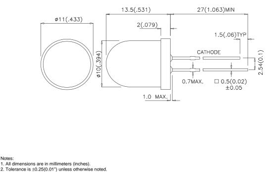
3. Lead spacing is measured where the leads emerge from the package.
