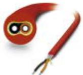
POF installation cable for fixed installation in the inner area with individual elements made of highly durable polyamide (PE). The cable is halogen-free, ozone and UV resistant and has a rugged polyurethane (PUR) outer sheath.
