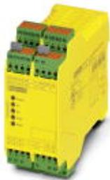
Safety relay for emergency stop and safety door monitoring up to SIL 3 or Cat. 4, PL e according to EN ISO 13849, automatic or manual activation, 3 N/O contacts, 1 N/C contact, 2 N/O contacts with fixed 3.0 s dropout delay, plug-in spring-cage terminal block
