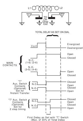
Applying voltage to the coil (for at least 50 msec) will transfer the switch, breaking the normally closed contacts (1-5 and 2-6), and making the normally open contacts (3-5 and 4-6). Contacts remain in this transferred position as long as the coil is energized. The time delay begins immediately upon de-energization. At the end of the delay period the switch returns to its normal position.
