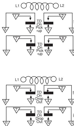
With the addition of an extra switch block at the bottom of the basic unit, this version of the Series 7000 offers four pole switch capacity with simultaneous timing or two-step timing. The two-step operation is achieved by factory adjustment to your specifications.
