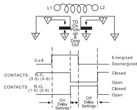
The Double Head model provides delayed switch transfer on energization of its coil, and delayed resetting upon coil de-energization. Each delay period is independently adjustable.
