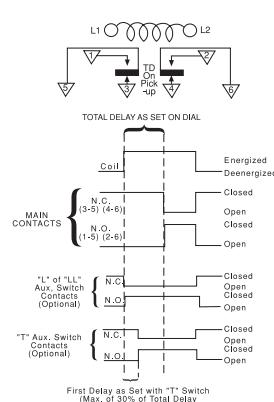
Applying voltage to the coil (L1-L2) for at least 50 msec starts a time delay lasting for the preset time. During this period the normally closed contacts (3-5 and 4-6) remain closed. At the end of the delay period the normally closed contacts break and the normally open contacts (1-5 and 2-6) make. The contacts remain in this transferred position until the coil is deenergized, at which time the switch returns to its original position.
