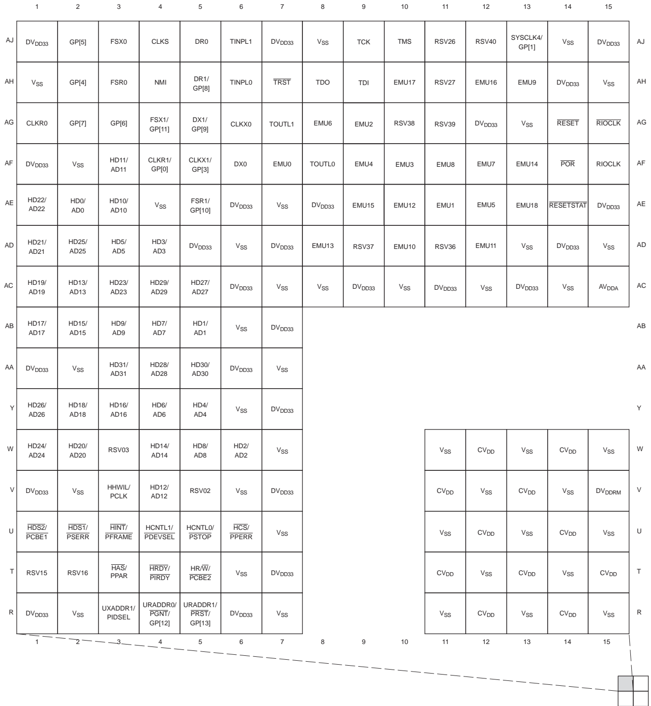
Figure 2-2. C6455 Pin Map (Bottom View) [Quadrant A]
