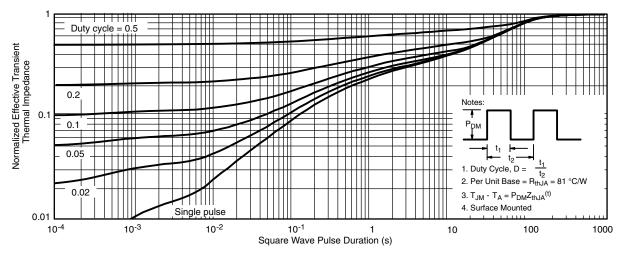
Normalized Thermal Transient Impedance, Junction-to-Ambient
