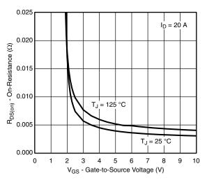
On-Resistance vs. Gate-to-Source Voltage
