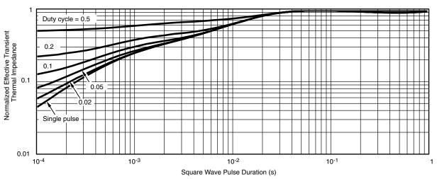
Normalized Thermal Transient Impedance, Junction-to-Case
